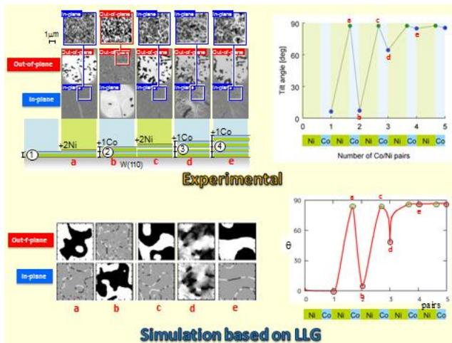
Fig.1 Magnetic domains of Co/Ni multi-layers
