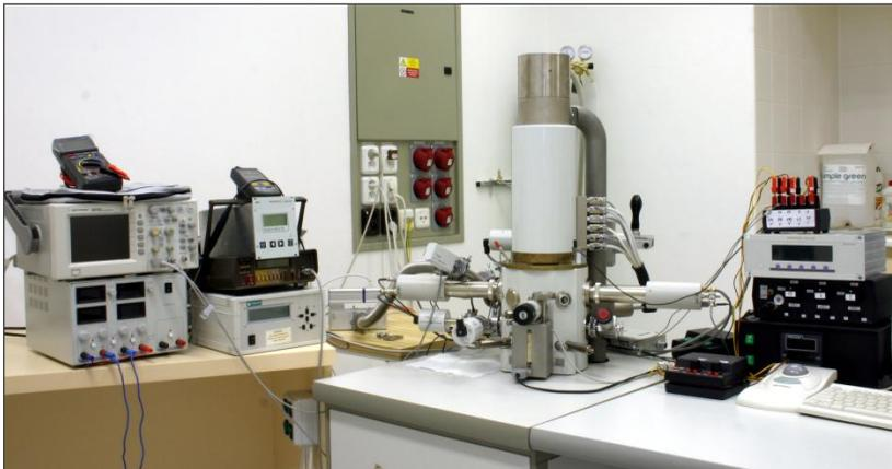
**Figure 1:** Environmental scanning electron microscope AQUASEM II.
