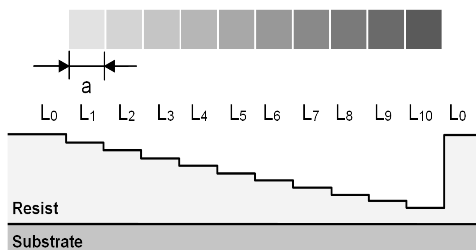
Figure 2: The model of relief structure for simulation created from ten lines ( a=1,0 \mu\text{m} ) exposed with linearly increasing dose.
