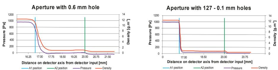
**Fig. 3:** Gas pressure and density dependence on detector axis for variant with one 0.6 mm diameter hole (left) and variant with 127 holes 0.1 mm in diameter (right).
