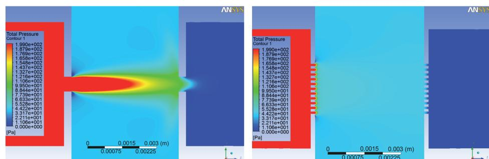
**Fig. 8:** Comparison of total pressure distribution for one-hole variant and for 127-hole variant.
