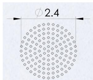
**Fig. 2:** Positioning of holes with diameter of 0.1 mm around centre of apertures A1 and A2.
