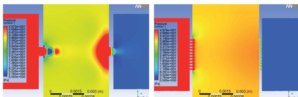
**Fig. 4:** Magnitude and distribution of static gas pressure in space between apertures A1 and A2. On left side is aperture with one hole (diameter of 0.6 mm) and on right side is aperture with 127 holes (diameters of 0.1 mm).
