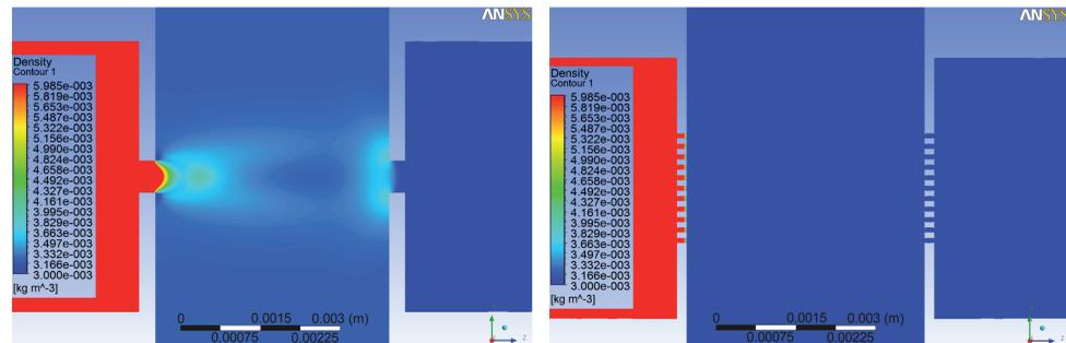
**Fig. 5:** Magnitude and distribution of gas density in space between apertures A1 and A2. On left side is aperture with one hole (diameter of 0.6 mm) and on right side is aperture with 127 holes (diameters of 0.1 mm).
