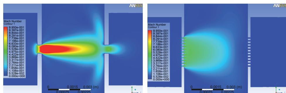
**Fig. 7:** Speed distribution characterized by Mach number for one 0.6 mm hole variant (left) and variant with 127 holes 0.1 mm in diameter (right).
