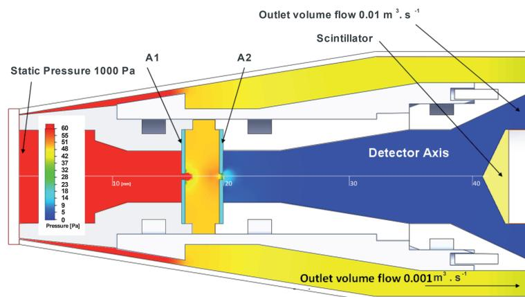
**Fig. 1:** Distribution of gas pressure in scintillation SE detector for ESEM (Inlet pressure 1000 Pa, pressure in scintillator chamber below 5 Pa, space between apertures A1 and A2 pumped by rotary pump with pumping speed of  $0.001 \text{ m}^3 \cdot \text{s}^{-1}$ , scintillator chamber pumped by turbomolecular pump with pumping speed  $0.01 \text{ m}^3 \cdot \text{s}^{-1}$ ).
